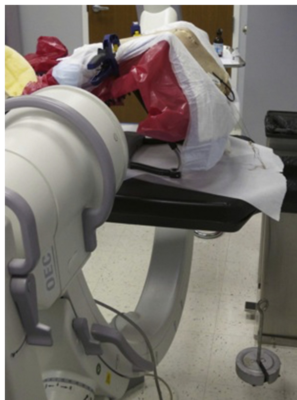
Fig 3. The knee was positioned in the continuous passive motion machine. Ten pounds of traction was added to the quadriceps tendon to stimulate an active extensor mechanism. Trochlear defects were cycled from a range of 0° to 40° of flexion, and medial femoral condyle defects were cycled from 0° to 120° of flexion.
