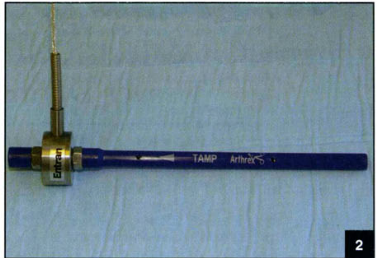
Figure 2. Modified tamp device holding a light weight 1 kN load cell (Entran).
