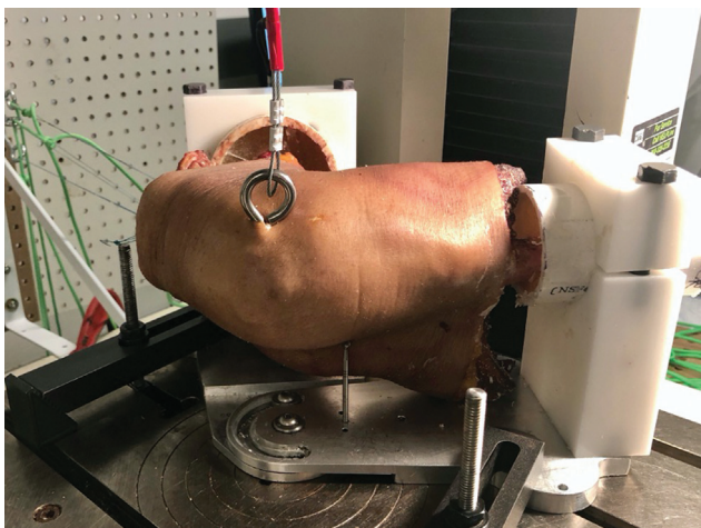
Fig. 2 Experimental testing setup. Photograph of a potted cadaver knee secured into a customized jig positioned perpendicular to the tensile testing machine that exerts its lateral patellar force vector through a steel cable connected to the lateral patellar eye screw.
