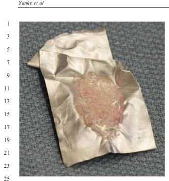
FIGURE 4. Fibrin being added to the DeNovo Natural Tissue in the negative mold.
