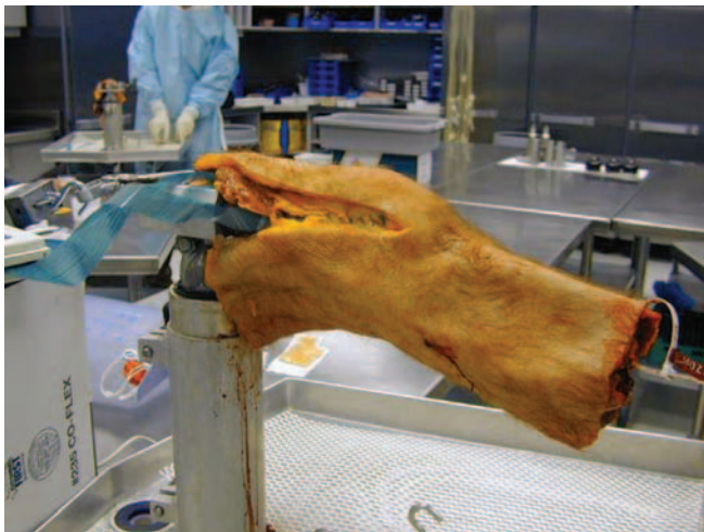
Figure 3. Testing apparatus with weight applied to the extensor mechanism.
