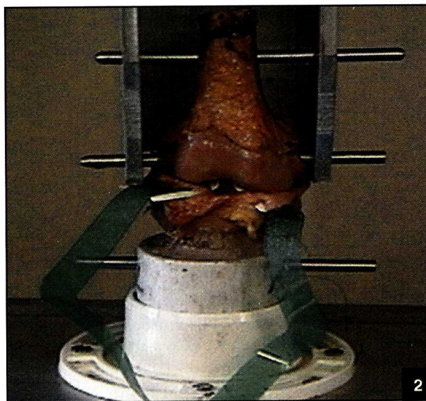
Figure 2. Sample specimen loaded in the Instron machine, with a K-scan sensor within the knee joint.
